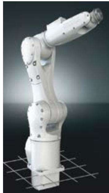
assistance are now possible. Positioned as a potential “third hand” for a service operator, the JoeBot is able to assist humans without the need for safety fencing. With a high Ingress Protection (IP) rating of 67 against solids and liquids, the JoeBot meets industry standards for use in both food and pharmaceuticals.<sup>10</sup>
